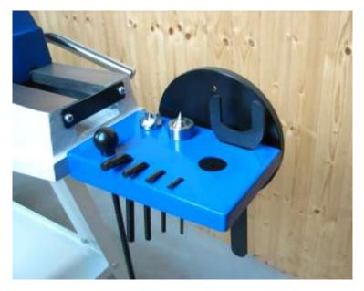
Bolt on the accessory storage tray using the 2 fixing bolts.
