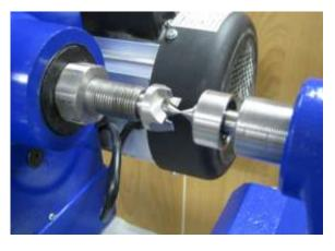
It is now necessary to check the alignment of the tailstock to the headstock. Fit both centres and slide the tailstock down towards the headstock until both centres touch and lock the tail centre in place. If the 2 centres do not meet correctly, undo the yellow headstock rotation locking lever and move the headstock slightly until the centres are aligned. Now lock the headstock.
