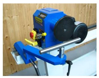
Bolt the left hand extension bed to the headstock end of the main bed using 2 fixing screws.
