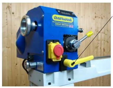
Fit the yellow lever onto the headstock locking shaft. Secure it in place with the spring and fixing screw. Tighten the fixing screw firmly.
