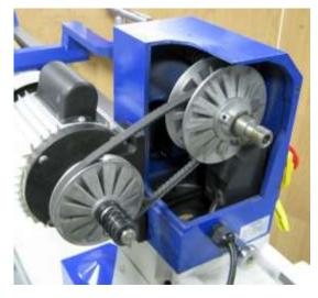
Over time the drive belt will become worn and will need replacing.
