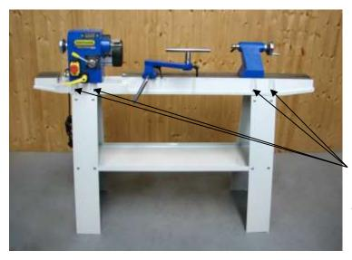
Lift (two people are required for this stage) the lathe bed, complete with headstock, tailstock and tool rest on to the stand (Fig. 2)
